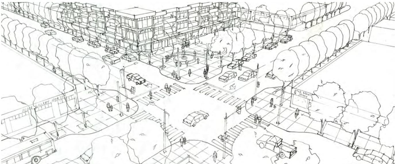
Plan and perspective views of 3-lane configuration at 100<sup>th</sup> St and 100<sup>th</sup> Ave intersection. This configuration would maintain significant through capacity and access while enhancing the pedestrian experience in the Downtown core area.
